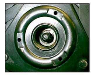
Should you receive a Delphi Harrison (GM) type compressor without the shaft nut, DO NOT attempt to install one. Attempting to install a nut on the shaft could alter the compressor clutch air gap.
