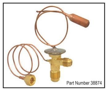
It is very difficult to determine if a Thermostat Expansion Valve is clean. The only way to be sure the valve is clean is to put it back into operation and run a system performance test. If there is any malfunction, the unit must be disassembled again to change the valve. It is more efficient to change the TXV as part of the compressor renewal.
