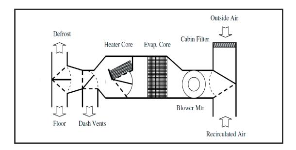
Note: If the vehicle does not have a cabin air filter, refer to TT329 Insufficient Airflow from Dash.
