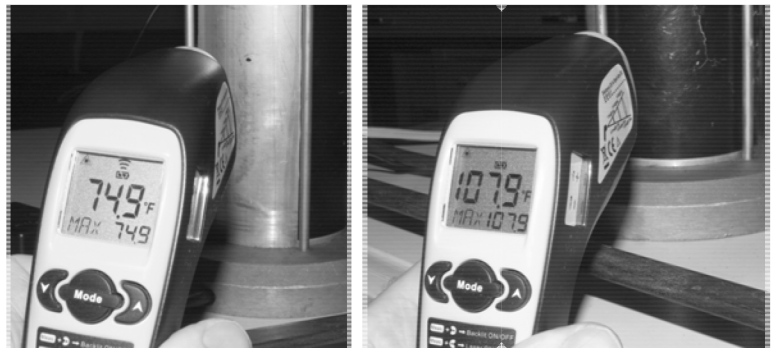
There “Appears” to be a 30 ° F Difference between the Bare Metal and Painted Surfaces – In Fact They are Both at the Same Temperature
