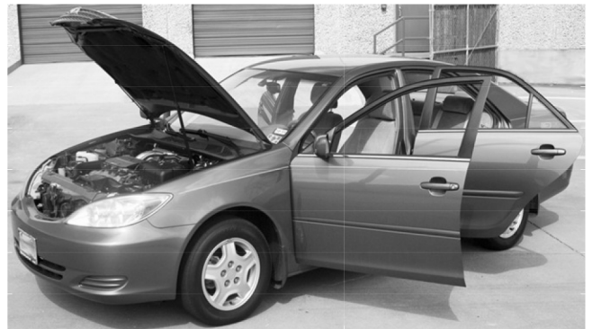
The Maximum Heat Load Temperature Test Is Performed Outside, In Direct Sunlight with Doors & Windows Open
