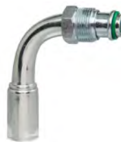
923111 Steel Male Insert O-Ring Hose Size: 10 Fitting Size: 10 Thread Size: 7/8" - 18
