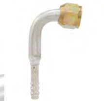
914906 Barb Fitting Hose Size: 6 Fitting Size: 6 Thread Size: 3/4" - 16
