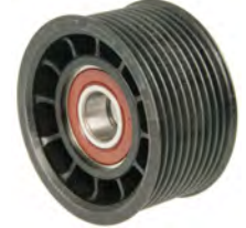
934156 Idler / Tensioner Pulley Serpentine Groove: 10 Pulley Dia.: 2-15/16 Belt Width: 1-9/16
