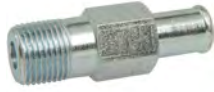
931300 Heater Fittings 5/8" Hose x 1/2" Male Pipe Thread - 2-1/2" Overall Length w/ Restricted Nipple
