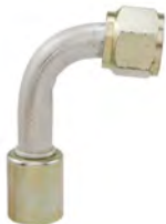
926904 Aluminum Beadlock Hose Size: 12 Fitting Size: 12 Thread Size: 1-1/16" - 14
