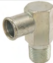
931345 Heater Fittings 3/4" hose to 1/2" NPT; w/hex fitting
