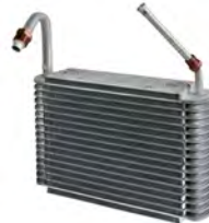
985107 Depth: 3-5/8" Height: 8-5/8" Width: 9" Inlet: Male Insert O-Ring Outlet: Male Insert O-Ring O-Rings: (1)[900208], (1) [900212]
