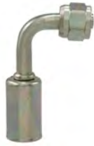
926911 Steel Beadlock Hose Size: 6 Fitting Size: 6 Thread Size: 5/8" - 18
