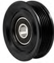
919318 Idler / Tensioner Pulley Serpentine Groove: 6 Pulley Dia.: 3-3/4 Belt Width: 1-1/4 FORD (10-02)
